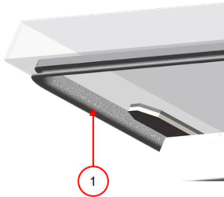
*Figure 28: Replacing the Lid Gasket*
