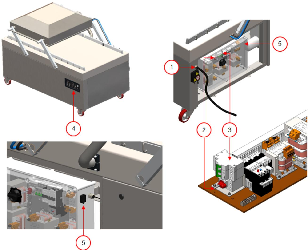
Figure 32: Overview of the Electrical Installation, Pampero, Solar
