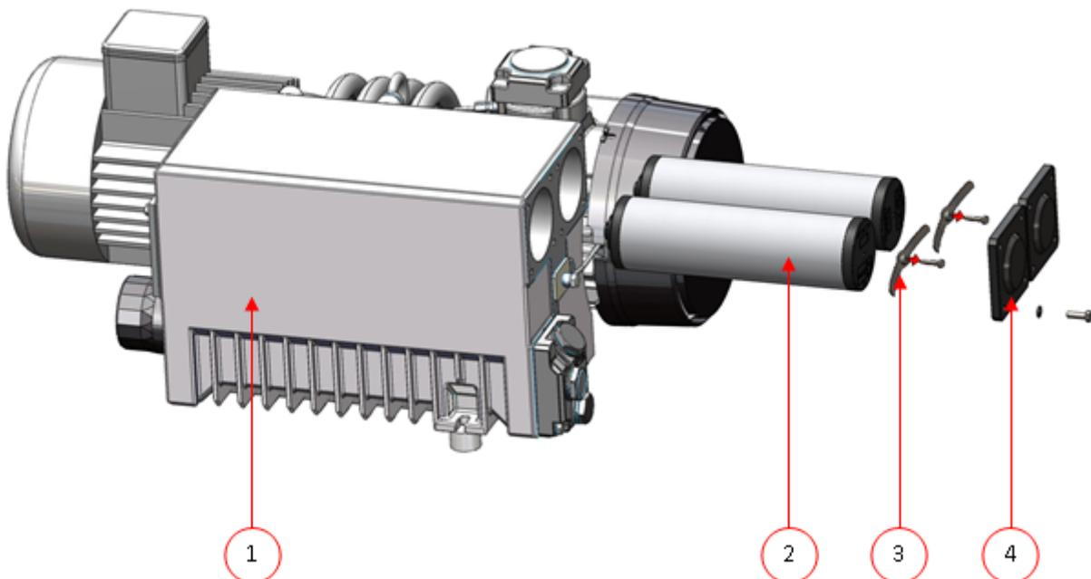
Figure 30: Replacing the Oil Exhaust Filter
