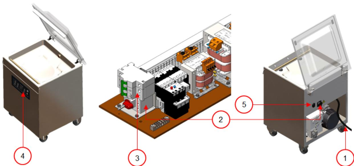
Figure 31: Overview of the Electrical Installation, Cyclone
