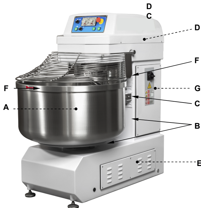
Figure 21 - Hazards of a mechanical and electrical nature characterising the machine
