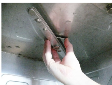
Remove the rinse arm on the top
