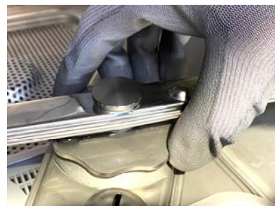
Daily assemble the lower rinse arm by working on the „big“ ring nut, like in the picture.
