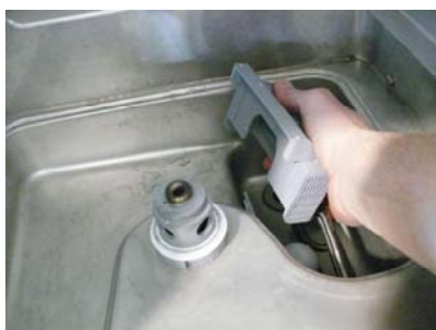
Remove the pump filter
