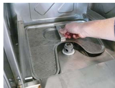
Remove the tank filters
