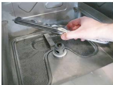
Replace the lower washing arm
