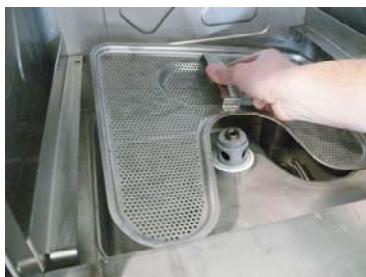
Insert the tank filter in its place
