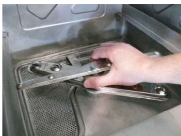
Unscrew the lower rinse arm
