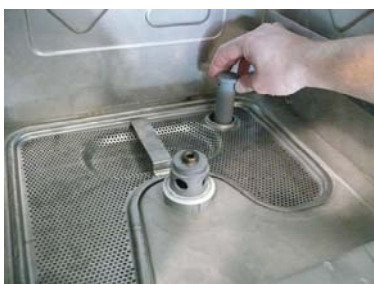
Remove the overflow pipe
