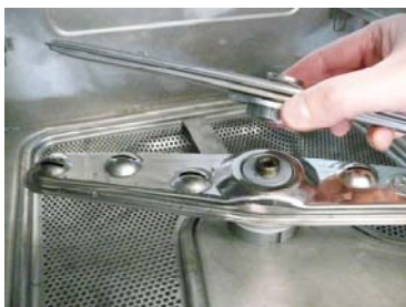
Replace the lower rinse arm
