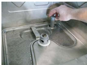
Replace the overflow pipe
