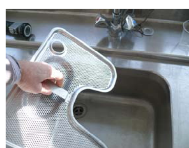
Clean the filter tank top
