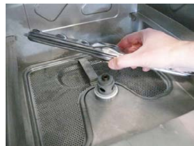
Remove the washing lower arm
