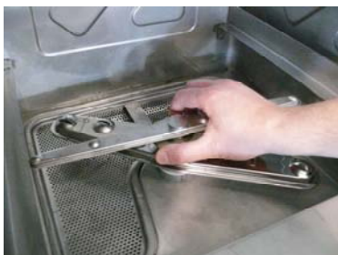
Unscrew the lower rinse arm
