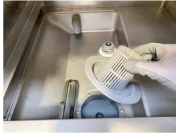
Remove the pump inlet filter
