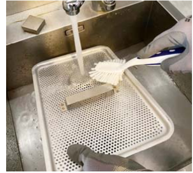
Clean the tank filter
