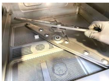
Remove the lower rinse arm
