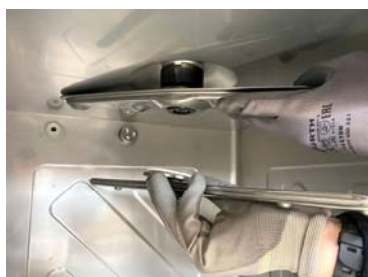
Remove the washing upper arm
