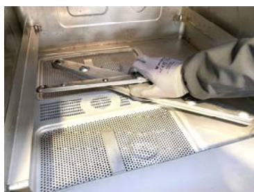
Unscrew the lower rinse arm
