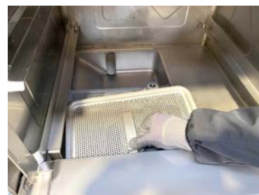
Remove the frontal tank filter
