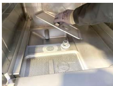
Remove the tank filters
