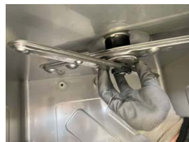
Remove the rinse arm on the top
