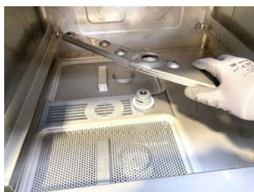
Remove the lower washing arm
