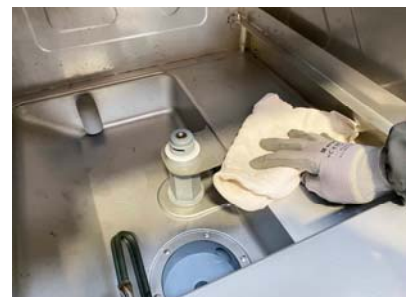
Remove from the tank by means of a brush or cloth if any, residual dirt.
