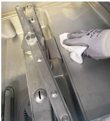
Clean the surface
