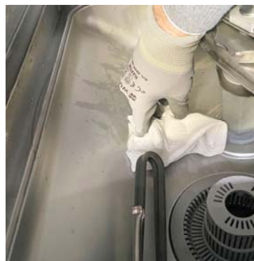
Remove from the tank by means of a brush or cloth if any, residual dirt.
