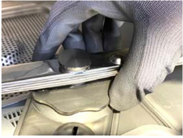
Daily disassemble the lower and upper rinse arms by working on the „big“ ring nut, like in the picture.
