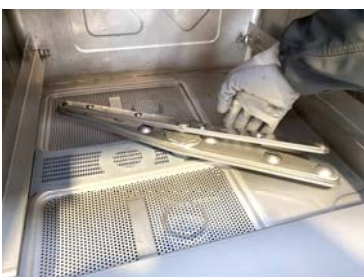
Check that the wash and rinse arms are free to rotate (upper and lower)
