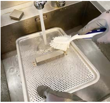
Clean the tank filters
