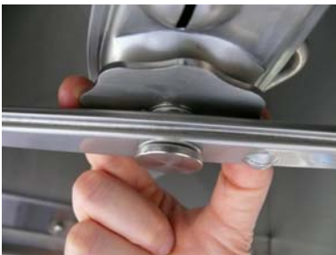
Unscrew the reel rinse top.
