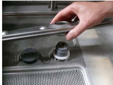
Remove the washing lower reel
