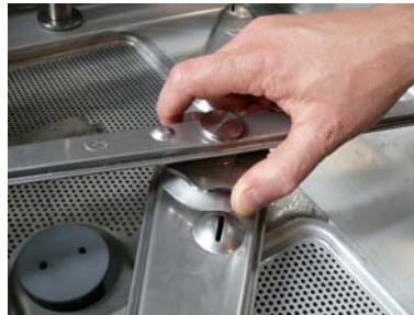
Unscrew the reel rinse lower
