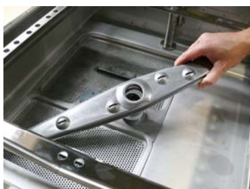
Replace the lower washing arm
