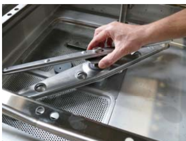
Screw the lower rinse arm
