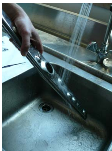
Clean the washing reel. Check for any debris inside.
