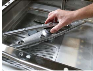
Screw the lower rinse arm
