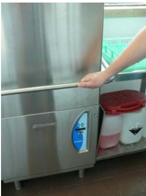
Completely close the hood the dishwasher. If there is an extended downtime, it is advisable to leave the hood open.
