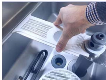
Insert the central support
