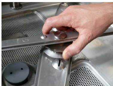
Unscrew the reel rinse lower
