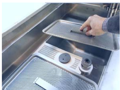
Remove the filters tank
