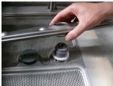
Remove the washing lower reel
