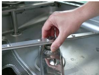
Unscrew the reel rinse lower
