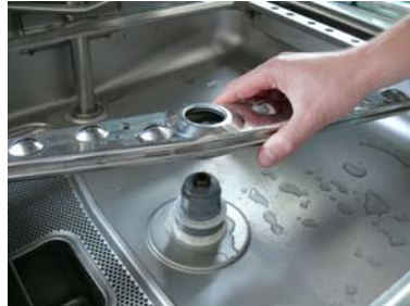
Remove the washing lower reel
