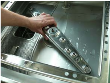
Replace the lower washing arm
