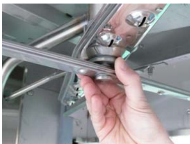
Unscrew the reel rinse top.
