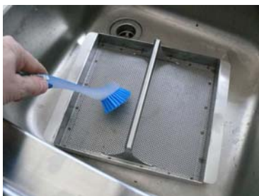
Clean the filter tank
