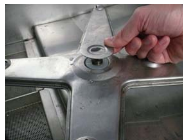
Replace the s.s. disc cod. 0800902 on the washing arm
