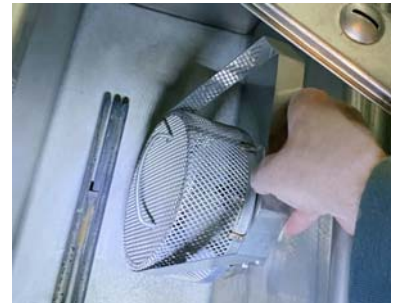
Insert the filter pump suction
