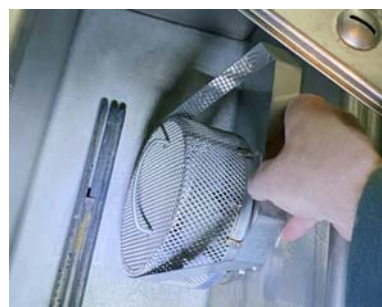
Remove the filter suction pump
