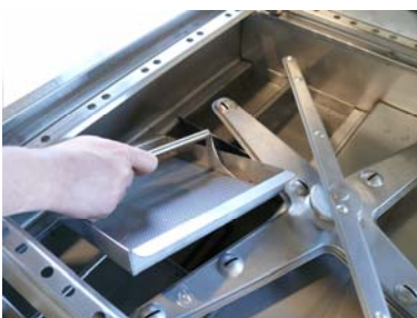
Insert the tank filter
