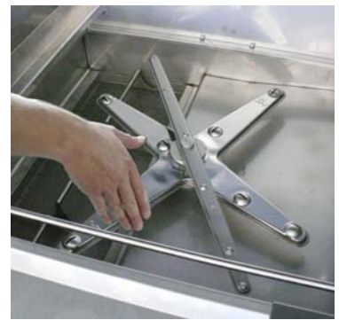
Check that the wash and rinse arms are free to rotate (upper and lower)
