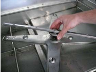
Screw the lower rinse arm
