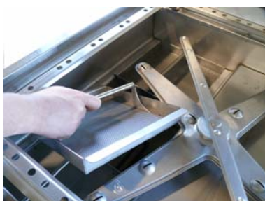
Remove the tank filters
