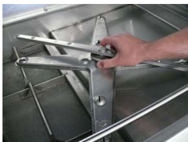
Unscrew the lower rinse arm
