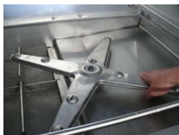
Replace the lower washing arm
