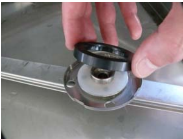
Control the wear washer cod.0201558 at the upper rinse arm is in his place.
