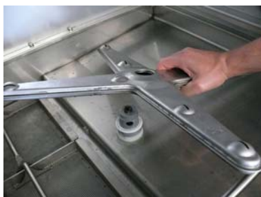
Remove the washing lower reel
