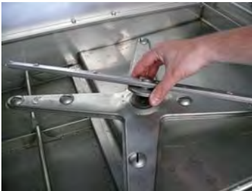
Screw the lower rinse arm
