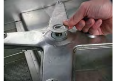
Replace the s.s.disc cod. 0800902 on the washing arm
