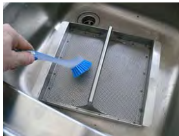
Clean the filter tank by means of a brush
