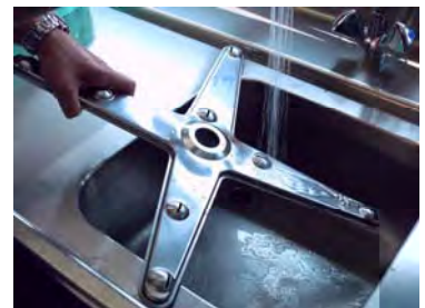
Clean the washing arm. Check for any debris inside.
