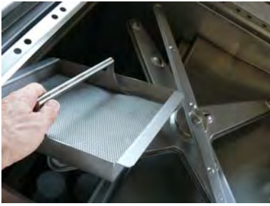
Remove all tank filters
