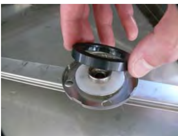
Control the wear washer cod.0201558 ot the upper rinse arm is in his place.
