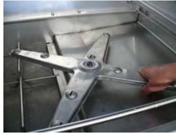
Replace tha lower washing arm
