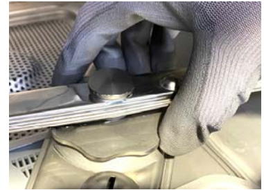
Daily disassemble the lower and upper wash arms by working on the „big“ ring nut, like in the picture.
