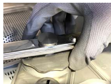
Daily disassemble the lower and upper wash arms by working on the „big“ ring nut, like in the picture.
