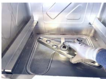
Replace the lower washing arm
