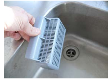
Clean the pump inlet filter by means of a brush
