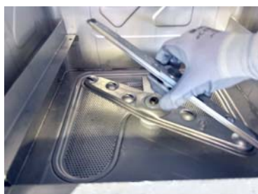
Replace the lower rinse arm
