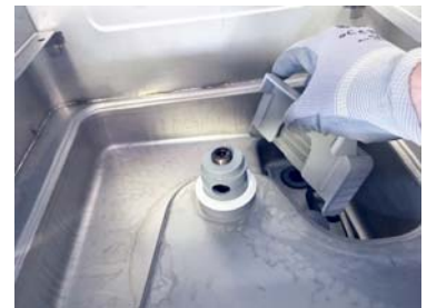
Then, at the end of the cleaning, insert the pump filter.
