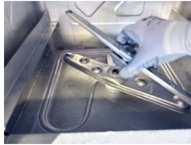
Unscrew the lower rinse arm
