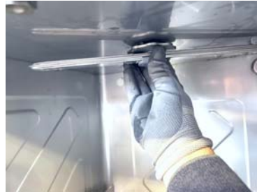
Remove the rinse arm on the top
